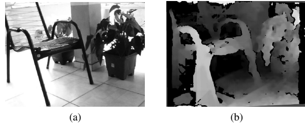
Fig. 3. An original scene and the corresponding disparity map, obtained by the technique. Original scene (a) Disparity map (b).
