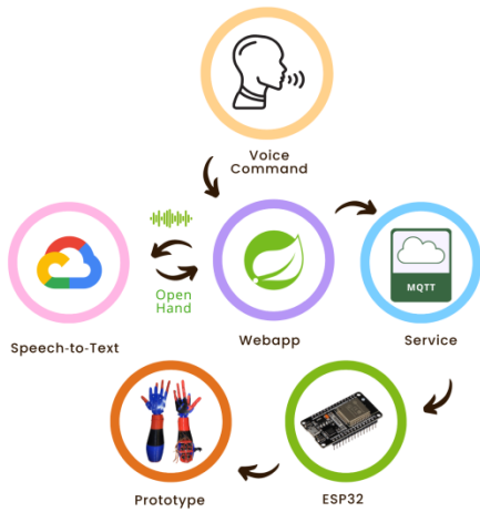
Fig. 2. Project's global communication architecture.
