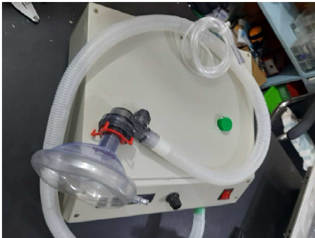
(a) Outside View; Dimension: 200mm x 200mm x 90mm; Weight: 1.6Kg.
