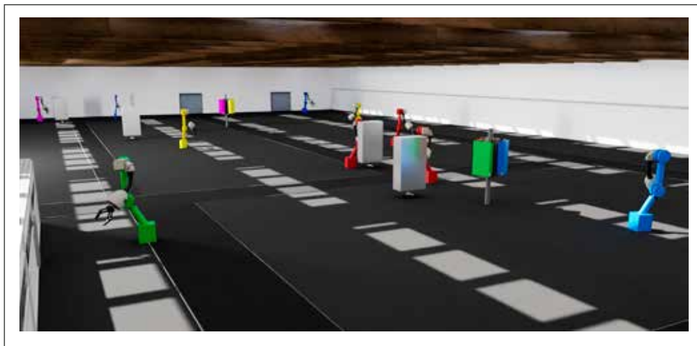
Figure 3 Illustration of a factory floor with 5G-connected stationary robotic arms and moving AGVs
