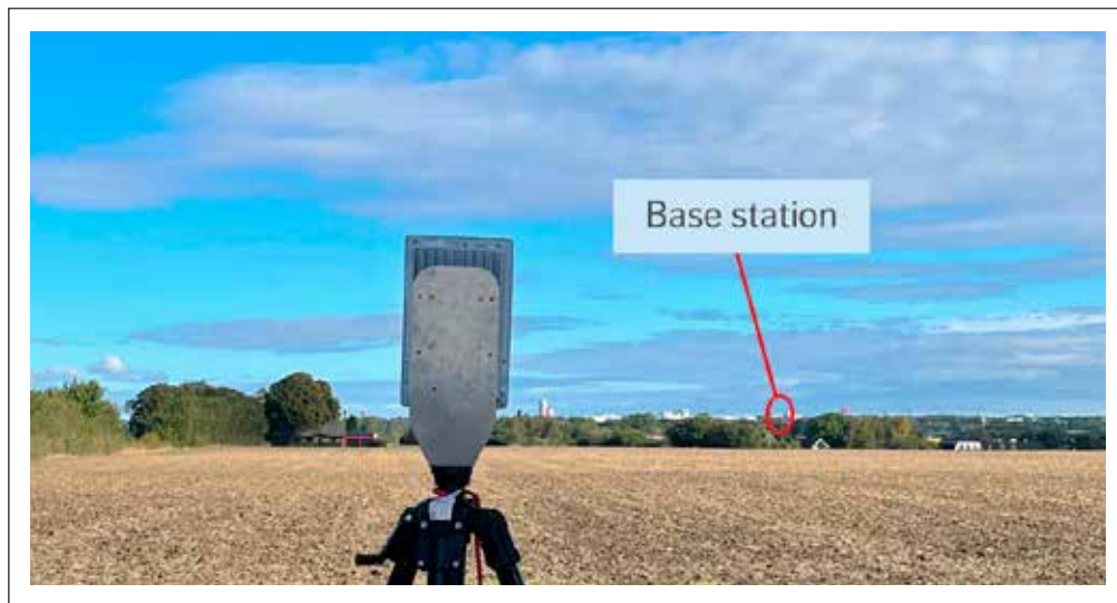
Figure 2 Testing of the mmWave extended range feature in a semi-rural area at a 6km distance from the macro base station
