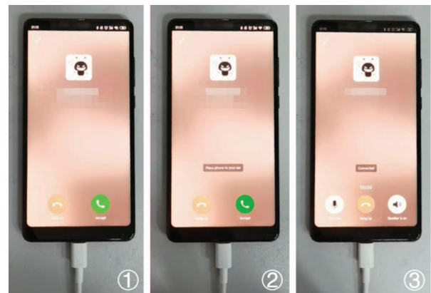
Fig. 27. Picking up an eavesdropping phone call. Step1: the attacker calls the victim; Step 2: the call is picked up by the ghost touches; Step3: the attacker can remotely eavesdrop on the conversations of the victims.
