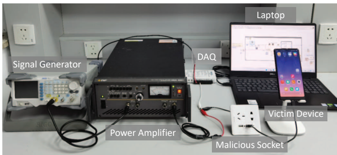
Fig. 18. Physical implementation of the attack system.
