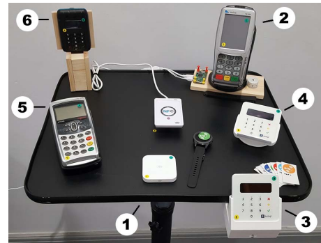
Figure 1: The equipment used in our experiment: six fixed terminals (labelled, see Table 1 for details), an NFC reader, a Raspberry Pi for timestamp collection, and a smartwatch.
