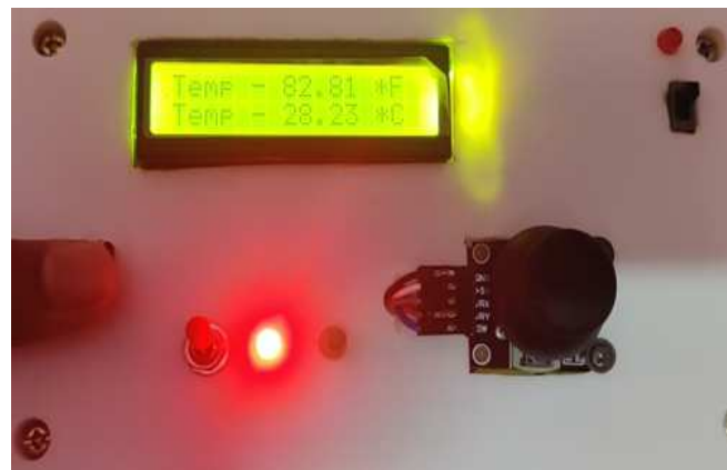
Figure 8: Transmitter Section of System with Temperature reading.
