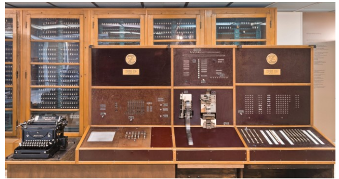
Fig. 1 The Z4 at Deutsches Museum. The console is visible in the foreground. In the background, we can see the racks of telephone relays used for the logic components. The two tape readers are visible in the center of the console. The right side of the console is used for entering instructions and addresses. The left side is used for entering decimal numbers, which are displayed in a lamp array similar to the keyboard of a vintage cash register. Results could be printed with the electric typewriter on the left.
