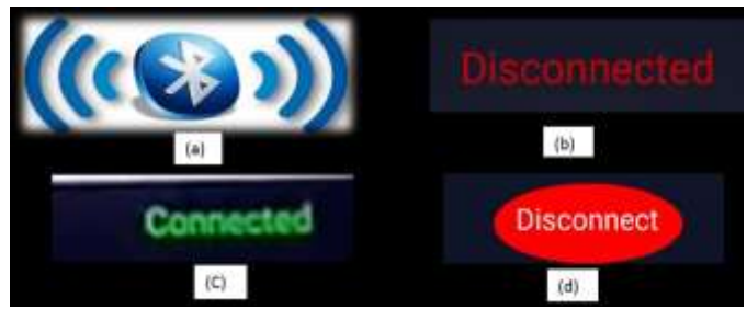
Fig. 10. Bluetooth link formation tab on mobile application: (a) Bluetooth Connect button (b) Text message showing Bluetooth not connected (c) Text message showing Bluetooth form pair with other devices (d) Bluetooth disconnect Button
