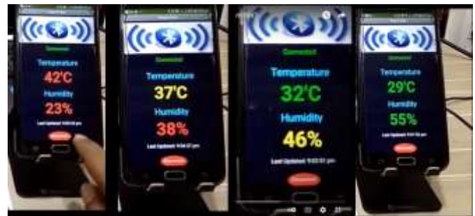
Fig. 8. Change of color of temperature and humidity parameters on mobile application
