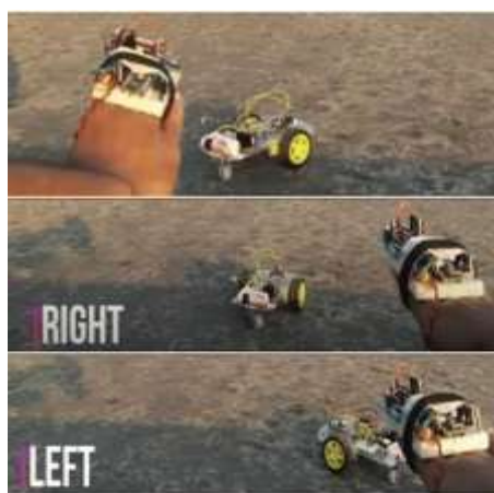
Figure-7: Sideways movement of the robot
