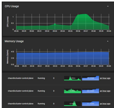
FIGURE 8. Memory usage remains relatively flat at less than 4 GiB, whereas CPU usage rises from its steady state of 0.25 cores to 1.3 cores during processing.
