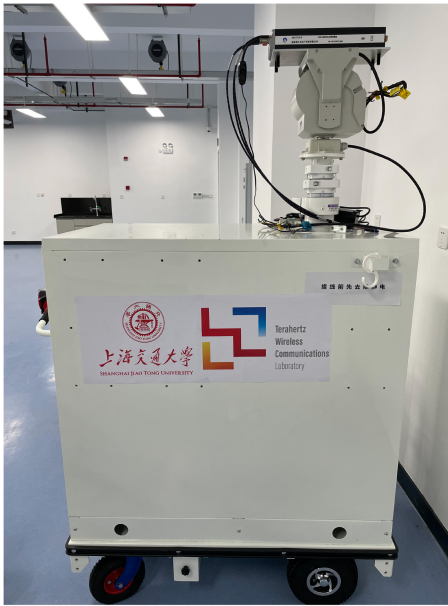
Fig. 3. The 260-400 GHz VNA-based channel measurement system.
