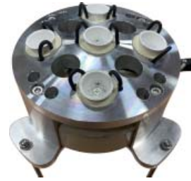
Fig. 26. LED transducer comprising five high-power LED segments and driver electronic individually pressure neutral potted.
