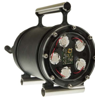
Fig. 27. Optical transceiver comprising five high-power LED arrays and a PD with a TIA circuit in the center. The transceiver is installed in a pressure housing with flat port (Fig. 23 (A)).
