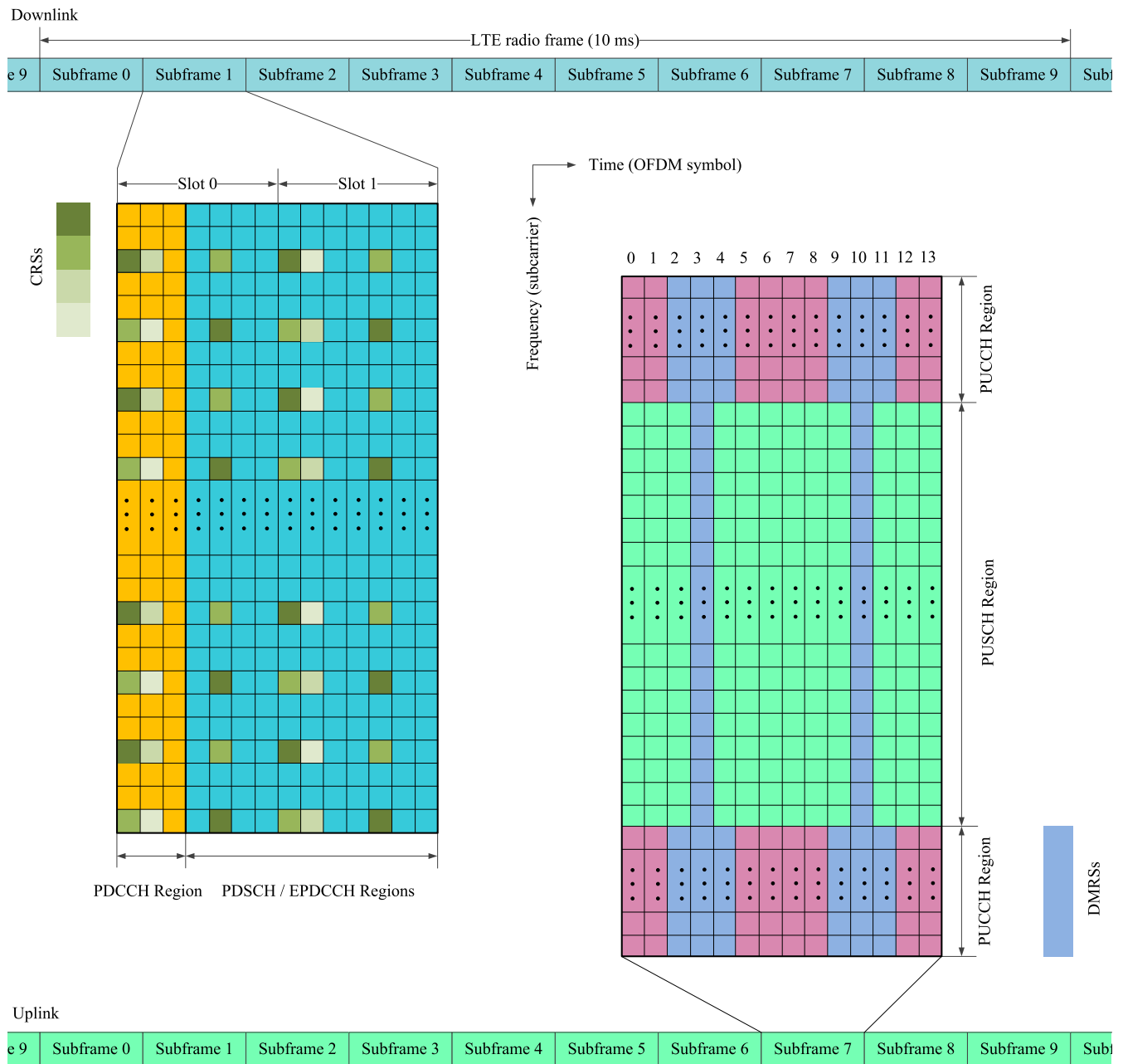
Fig. 2. Illustration of LTE frame structure, in which the transmission follows a continuous and deterministic time line that consists of a sequence of contiguous radio frames. A radio frame contains 10 subframes, each of which is composed of 14 OFDM symbols (i.e., two slots). The first up to three OFDM symbols of a downlink subframe are used for control channels like PDCCHs and PHICHs, and the remainder is primarily for downlink traffic (PDSCHs). The enhanced PDCCHs (EPDCCHs) can also be frequency-division-multiplexed with PDSCHs. The two end parts of an uplink subframe in frequency domain are used for PUCCH, while the rest is for uplink traffic (PUSCHs). DMRSSs are demodulation reference signals.
