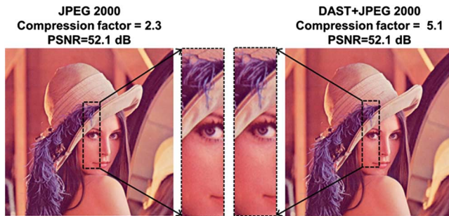
Fig. 5. Performance of Discrete Anamorphic Stretch Transform (DAST). Left column: image compressed by JPEG 2000. Right column: image pre-compressed using DAST followed by JPEG 2000. In both cases the decoded image PSNR is 52.1 dB but the case with DAST pre-compression has more than twice compression factor.
