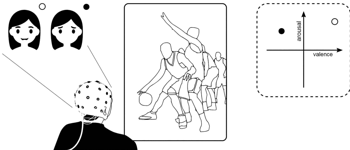
FIGURE 1. An affective dimension of relevance enables computing systems to interpret users' emotional and affective responses, in addition to conventional measures of relevance or interest. In the scenario depicted in the figure, a user watches a basketball game. User signals, such as brain recordings or facial expressions, can be used to determine which affective reactions the content evokes in the user. For example, depending on whether a user is a fan of a winning team (positive valence marked with a white dot) or a fan of a losing team (negative valence marked with a dark dot), the same relevant and interesting (high arousal) content can evoke different affective reactions.
