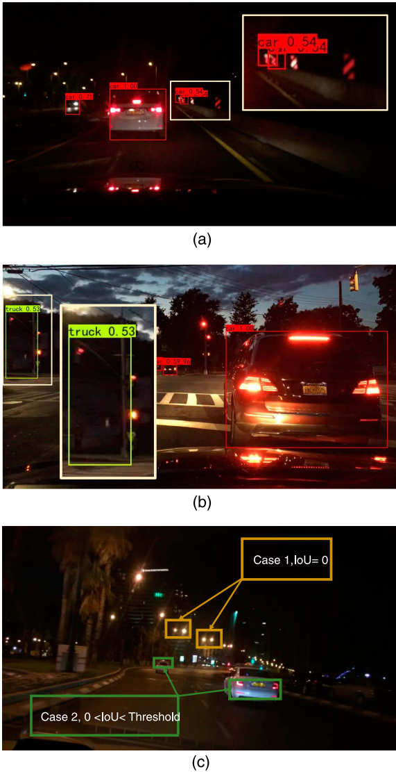
FIGURE 3. Illustration for the false detection cases. (a) and (b) Examples of false detection due to disturbance from interfering light sources. (c). Cases for the detected background proposals that may be misclassified during training.
