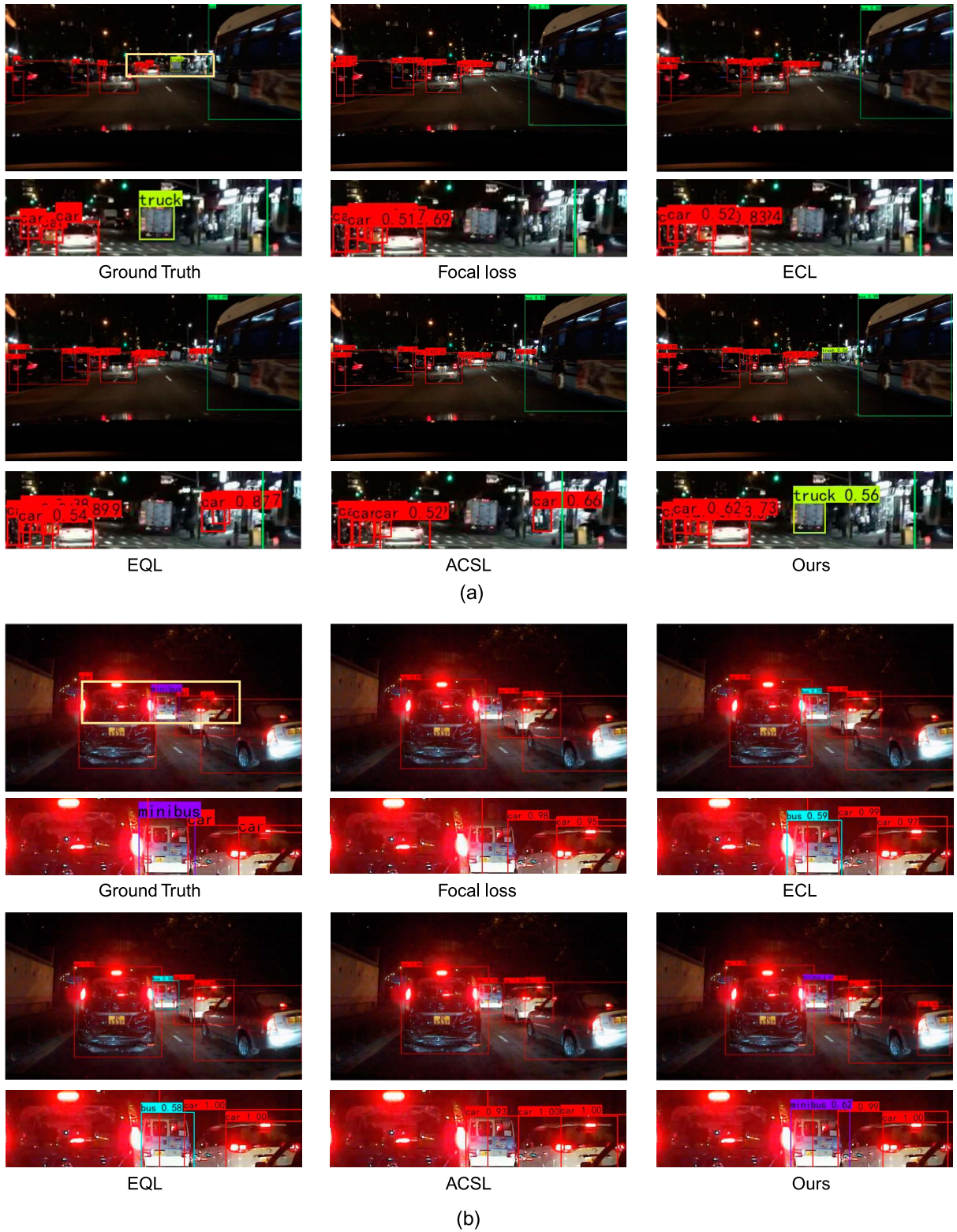
FIGURE 4. Visual comparison of the results from the baseline model using each method for nighttime vehicle detection.
