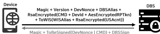
Fig. 3. Secure protocol in the registration phase is illustrated.
