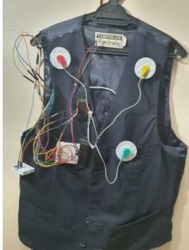
Fig. 8. Hardware setup of the portable health monitoring system
