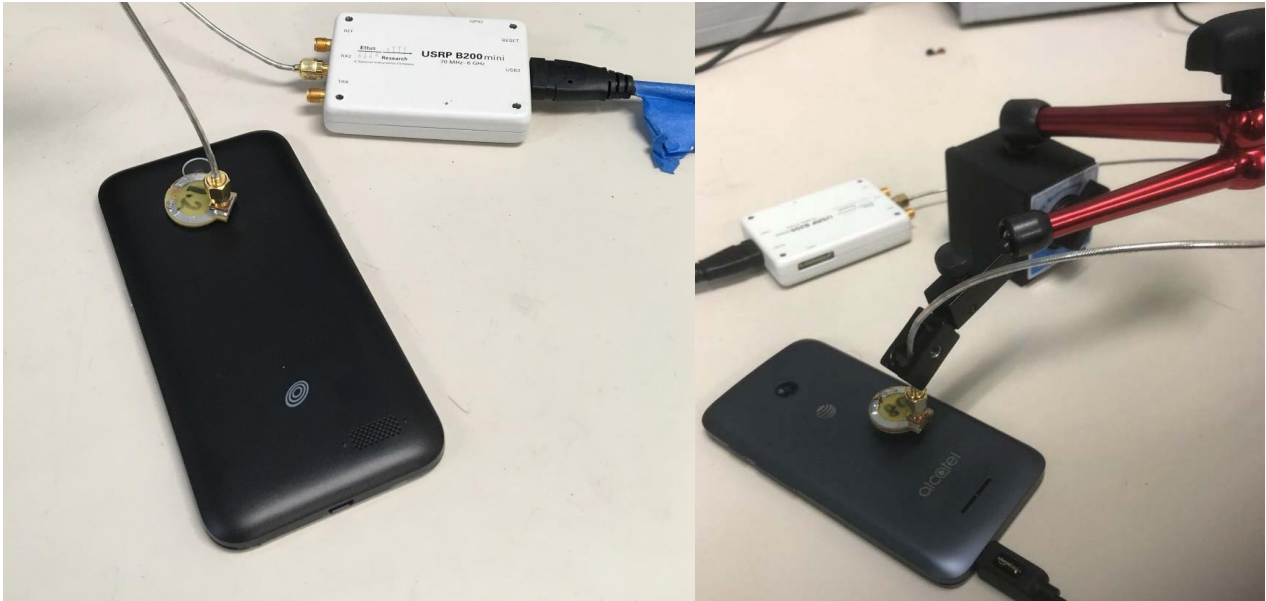
Figure 1. Experimental setup for capturing EM emanations from ZTE ZFIVE (left) and Alcatel Ideal (right) phones. In each setup, our custom probe (the flat, beige, circular object at the end of the silver-colored cable) is positioned close to but not touching the phone. The cable is held in position by a mechanical arm, which is visible in the photo on the right. An Ettus B200-mini SDR (white box) digitizes the signal and sends it through a USB cable to a personal computer (not shown) for analysis.
