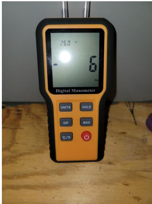
FIGURE 11. Modified digital manometer reading the static pressure in an HVAC system.
