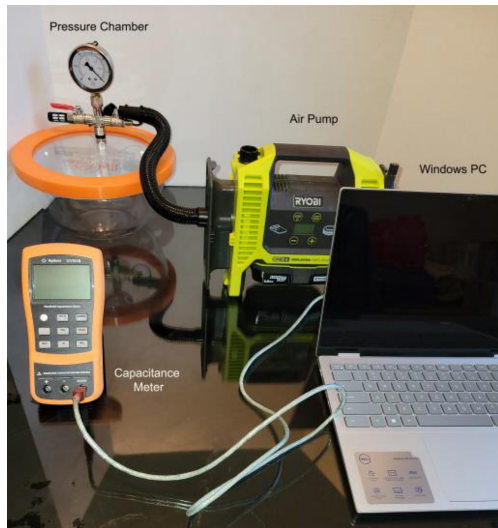
FIGURE 7. Experimental setup: pressure chamber, air pump, capacitance meter, and a Windows PC.
