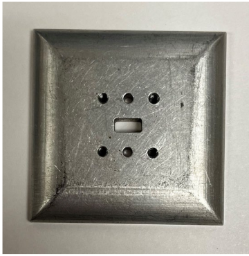
FIGURE 15. Picture of a Ka-band modified open-ended rectangular waveguide flange based on the design in [18].
