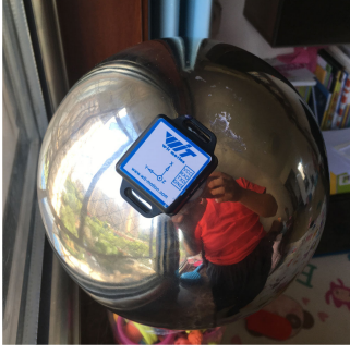
Fig. 4. Hollow steel ball and IMU sensor. The IMU sensor is fixed on the hollow steel ball.
