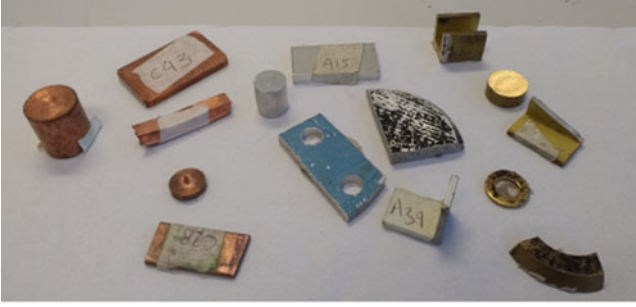
Fig. 5. Subset of typical test pieces. A total of 117 test pieces are used in copper (36 pieces), aluminum (44), and brass (37).
