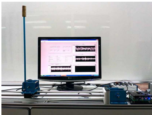
Fig. 10. Linear inverted pendulum used in the testbed.
