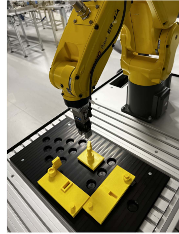
Fig. 2. Experiment setup representing a common pick-and-place operation in a robotic manufacturing.
