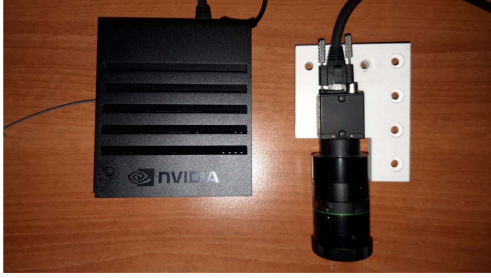
Fig. 5. Proposed setup consisting of a Jetson AGX Xavier and a machine vision camera.
