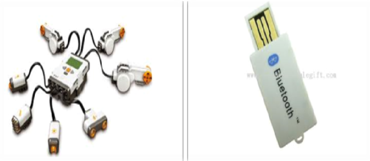
Figure 2. At Left: Lego NXT Controller units connected with different sensors, At Right shows the Bluetooth dongle used with the system for wirelessly controlling the whole system.
