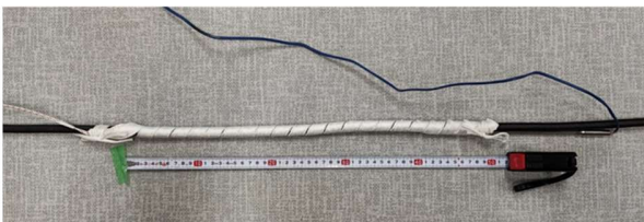
Fig. 4. Photo showing the partial heating method by wrapping a ribbon heater.
