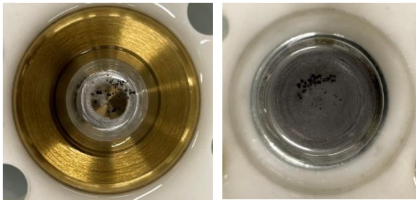
Fig. 19. Electrode breakdown marks requiring sand-polishing.
