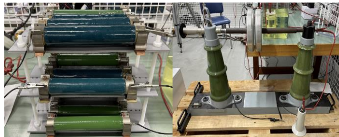
Fig. 16. Left: Resistance bank ( R_t ) Right: HV disk capacitor ( C_t ).
