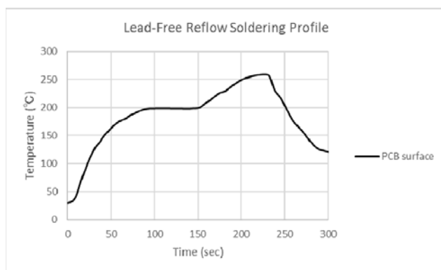
Figure 5. Lead-free reflow soldering temperature profile.
