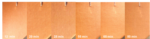
Figure 10. Surface tracking process on a wet pressboard surface (moisture content: 4.3%) in Gemini X at 50.0 kV.
