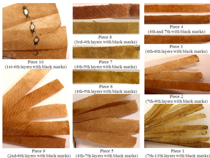
Figure 18. Tree-shaped carbonized mark inside the layers of the vertical pressboard stressed for 3 hours at 43.0 kV and 6 hours at 55.0 kV in MIDEL 7131.
