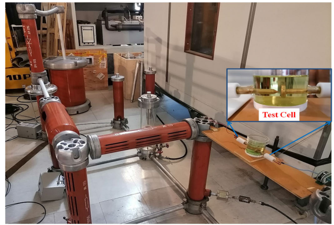
Fig. 1. Test setup and the custom-made test cell for lightning impulse voltage test setup.
