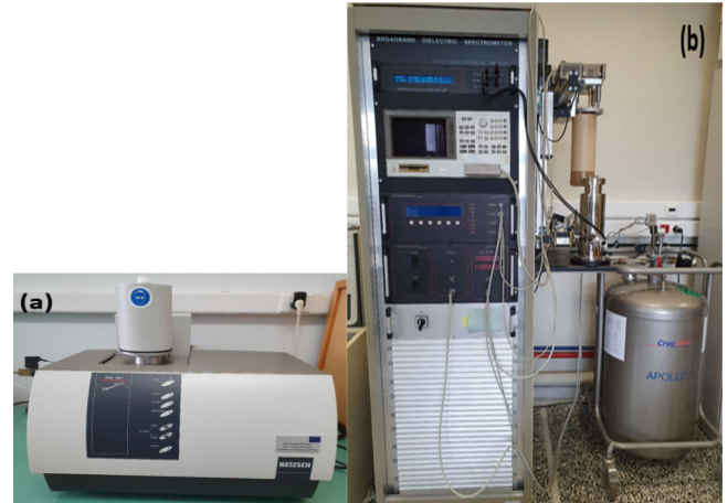
Fig. 2. Apparatuses used for thermal diffusivity and relative permittivity measurements. (a) NETZSCH LFA 467 Hyper Flash device. (b) Novo-control Alpha analyzer.
