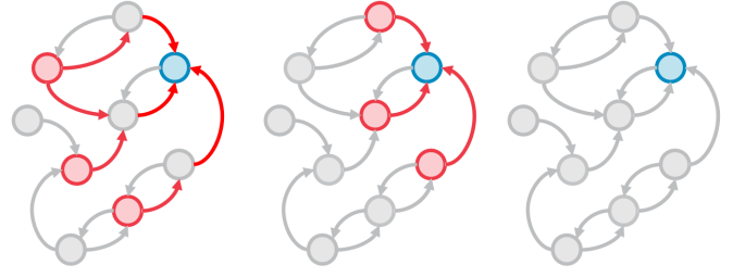
Fig. 1: TAGCN Polynomial filter of degree 2 for blue node, signals at the red nodes are propagated to the blue one and aggregated, i.e., \mathbf{A}^2 x^{(\ell)} \mathbf{W}_2^{(\ell)} + \mathbf{A} x^{(\ell)} \mathbf{W}_1^{(\ell)} + \mathbf{I}_N x^{(\ell)} \mathbf{W}_0^{(\ell)}
