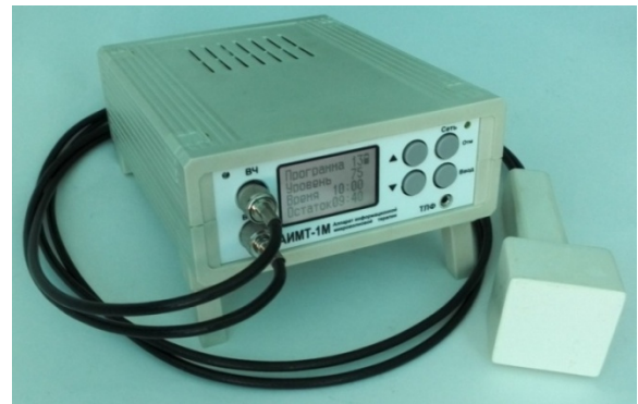
Fig. 1. The device for modeling the solar microwave radiation
