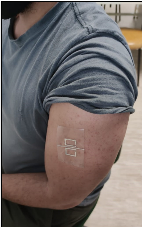
Fig. 4. RFID tattoo attached to a human arm.
