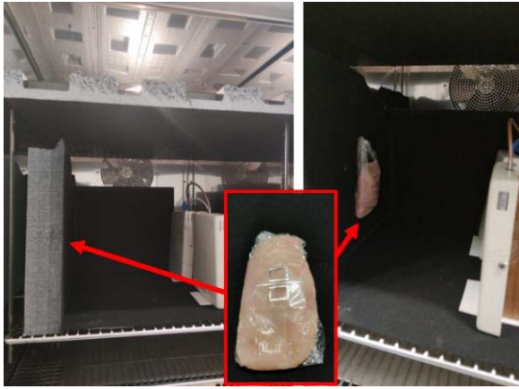
Fig. 7. Internal view: Setup of Temperature Variation in a Climatic Chamber using a chicken breast.
