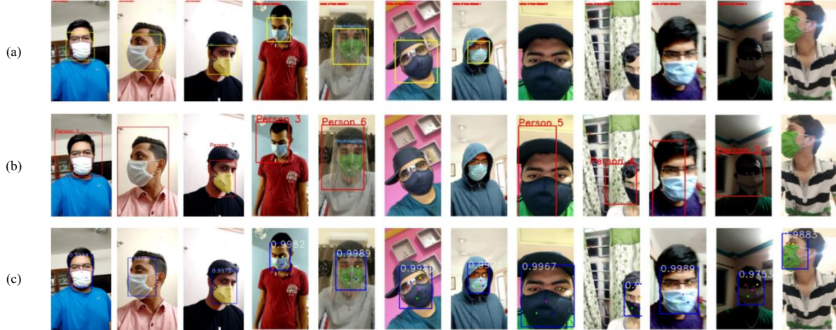
Fig. 5. Detection results of different algorithms on the dataset video frames. (a) YOLO-face. (b) YOLOv3. (c) RetinaFace.
