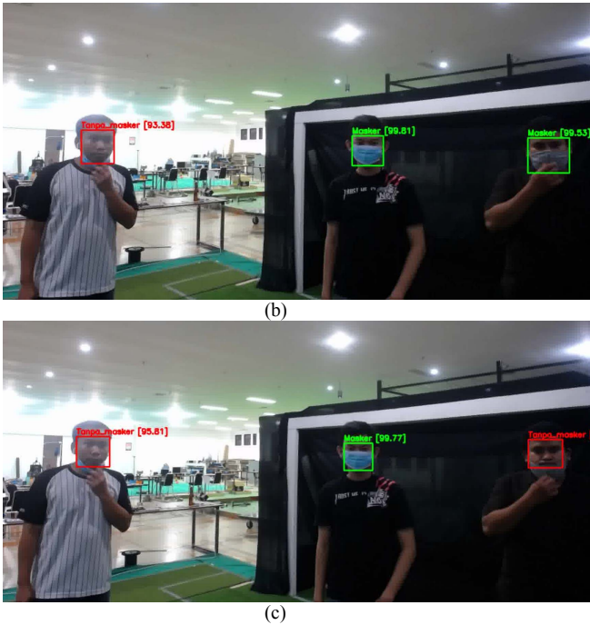
Fig. 6. The face mask detection detected the non-wearing user with different angle of pose.
