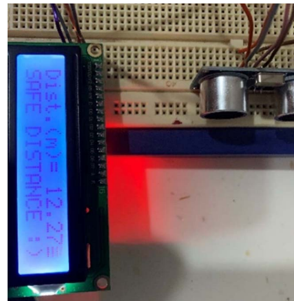
Fig. 9. The message displayed on the LCD when the subject is at a distance more than 1 metre
