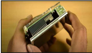
Fig. 4. Connection of TFT and Raspberry Pi 4
