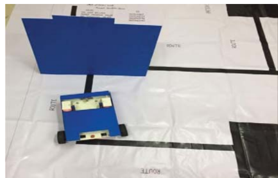
Fig. 12: Sensing the obstacle, it stops and denies to move towards
