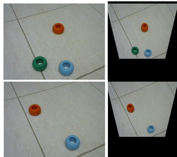
Fig. 3: Sample frames of the custom dataset and their respective bird's eye view transformation
