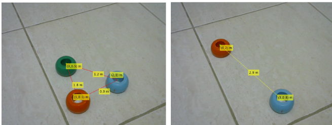
Fig. 9: Locations and distances in real-world coordinates of the custom dataset. Where intentionally, 10cm in real-world is treated as 1m.
