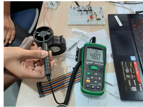
Fig. 3. Reverse engineering airflow measurement without HE filter
