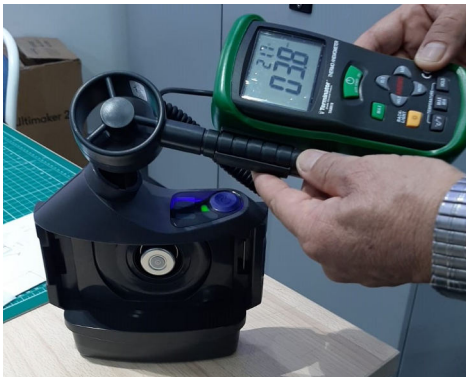
Fig. 2. Original devices airflow measurement without HE filter
