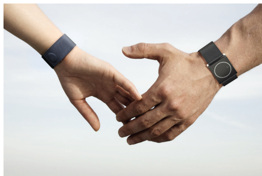
Figure 3. The Empatica Embrace wristband measures multiple physiological signals and can run apps to detect and communicate autonomic stress and movement patterns, potentially saving lives.
