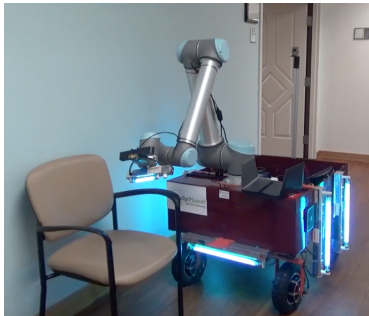
Fig. 3. Proposed virus disinfection robot
