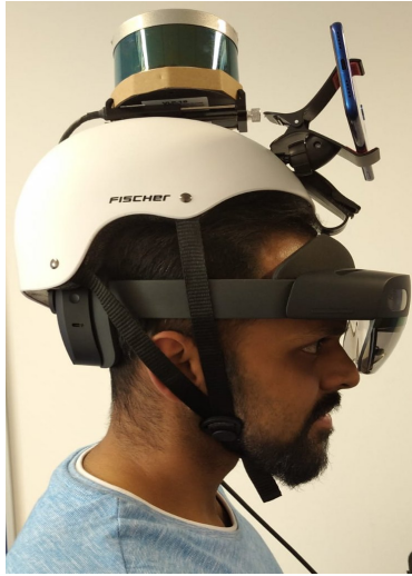
Figure 2: (a): Pedestrian with the social distancing helmet, (b): Different components of the SDH interacting with the system
