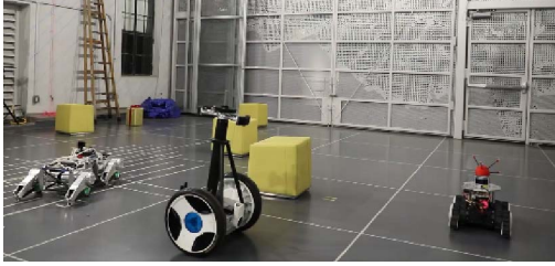
Fig. 4. Three robots involved in experimental evaluations at CAST: (left) quadruped, (center) Segway, and (right) Flipper.
