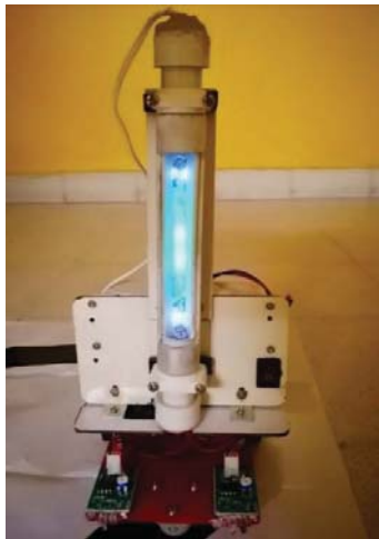
Fig. 7 100% exposure of Far UVC.207-222 nm light to its surroundings as controlled by the UV C light cap
